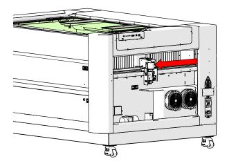
Loosen, but do not remove the four (4) Phillips screws that hold the x-axis motor drive board cover:
