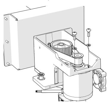
Install the x-axis reducer belt:
