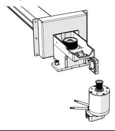
The x-axis encoder connection must face the front of the engraver as shown above. Any other orientation will prevent the engraver from booting up properly.
