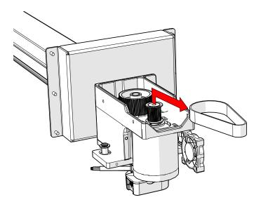
Remove the four (4) 2.5mm Allen screws that secure the x-axis motor to the x-axis assembly:
