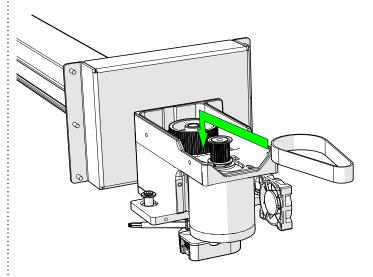
Apply tension to the x-axis reducer belt by pulling the motor away from the x-axis reducer pulley. Once the slack is removed from the reducer belt, fully tighten the four (4) 2.5mm Allen screws that hold the x-axis motor to the x-axis assembly.
