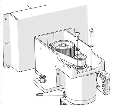
Remove the x-axis motor:
