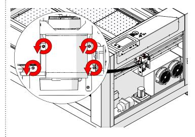
Remove the x-axis motor drive board cover.
